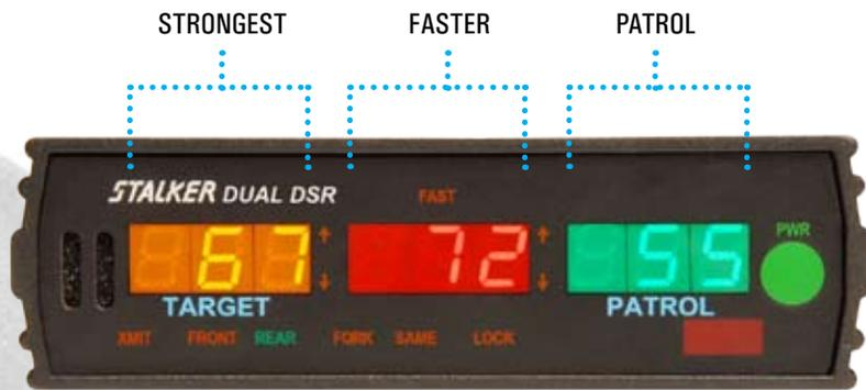
*By displaying both strongest and faster targets simultaneously, the Stalker DSR can monitor faster vehicles passing larger vehicles and display the speed of both targets simultaneously.*
