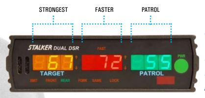
By displaying both strongest and faster targets simultaneously, the Stalker DSR can monitor faster vehicles passing larger vehicles and display the speed of both targets simultaneously.
