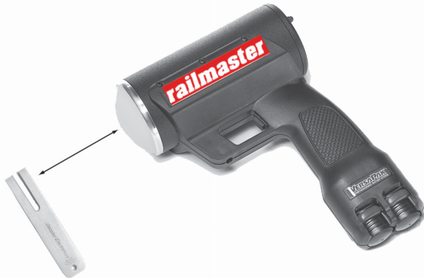
Figure 6.1 Place the vibrating tuning fork about 3 inches in front of the antenna.
